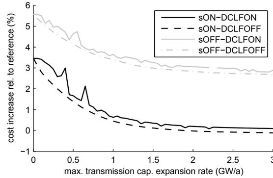
Figure 10: Sensitivity analysis for max. transmission expansion rate and DCLF constraints. Overall costs are affected by power flow distribution modeling, but the effect is smaller than that constraining transmission and storage availability.
