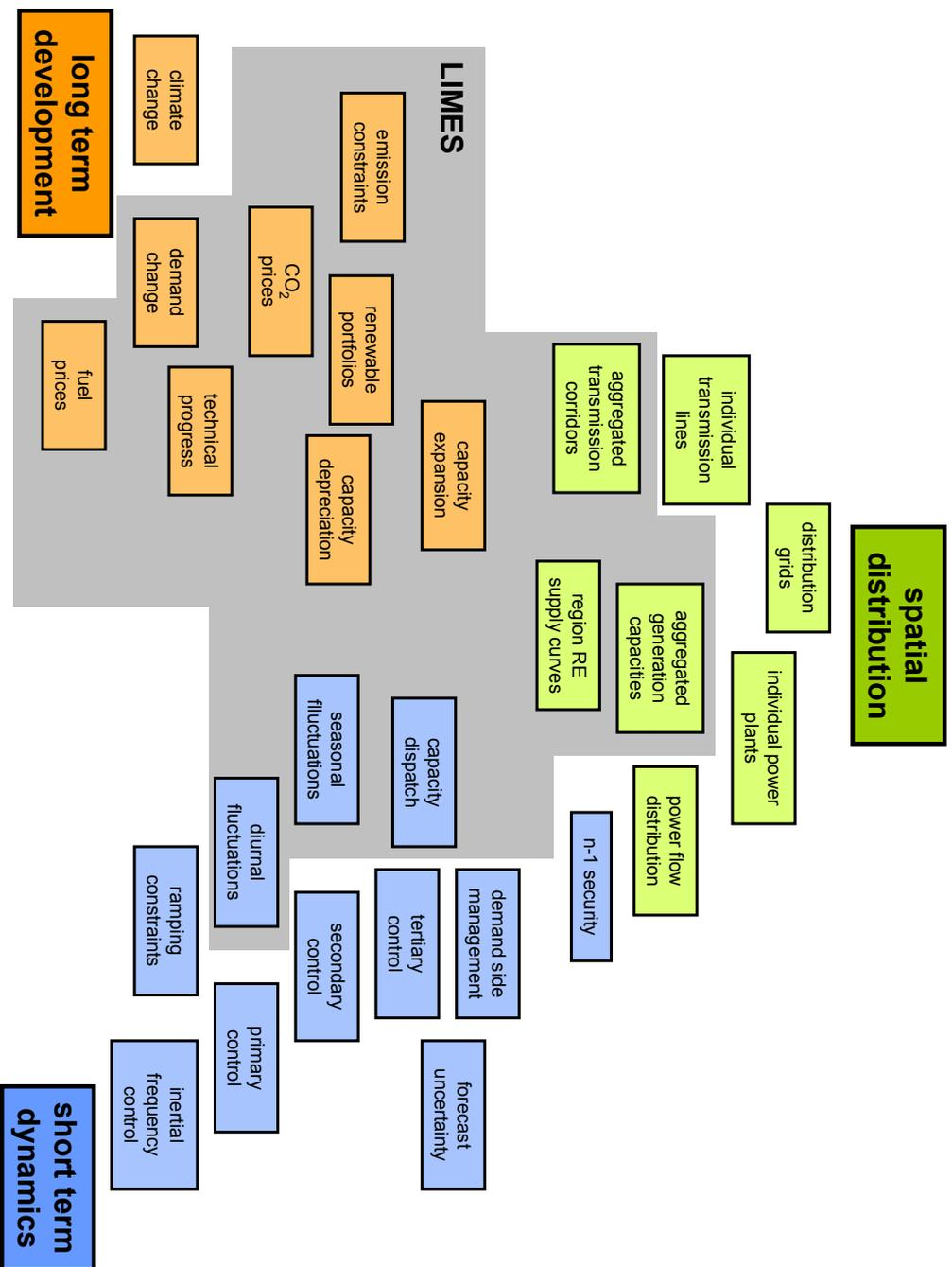
**Figure 1.5:** System integration of fluctuating renewable energy: overview of challenges. The shaded area marks the challenges that are taken into account by the LIMES model.
