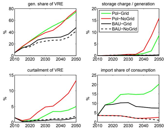
Figure 4: Long term system development for all scenarios. The panels show generation share of fluctuating RE, storage charge to total generation ratio, import to total consumption ratio, and curtailments of fluctuating RE.
