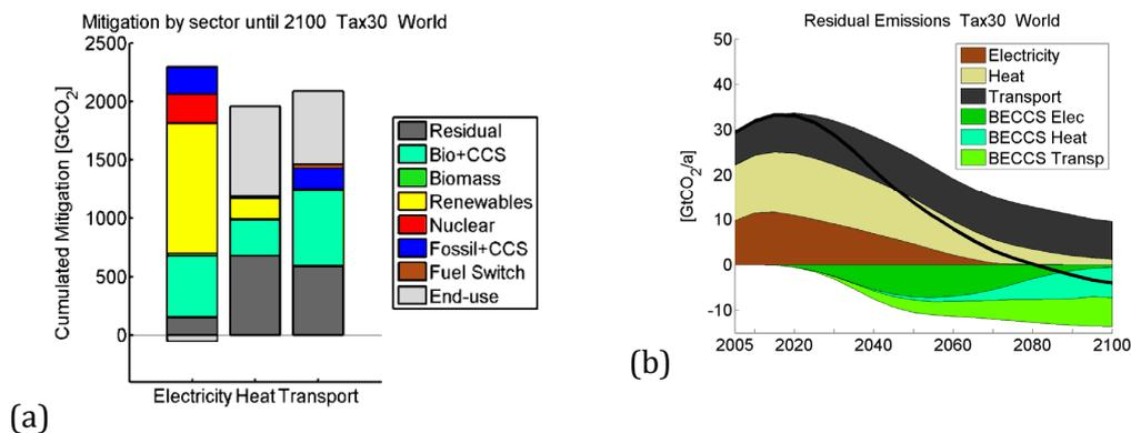
**Figure 3: (a) Mitigation contribution of technologies cumulated from 2005-2100, and broken down by the end-use sectors electricity, heat, and transport for the TAX-30 climate policy scenario. (b) Residual emissions decomposed by end-use sector. The solid black line in (b) indicates net emissions.**
