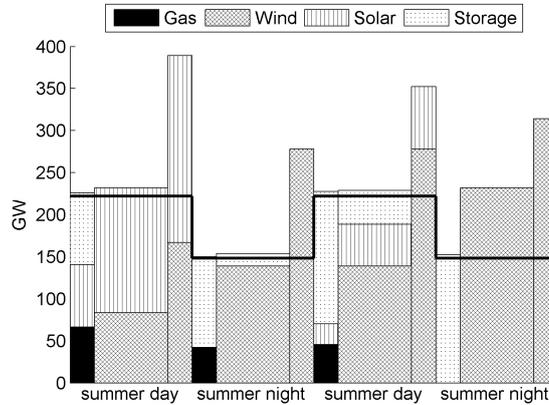
Figure 3: Global generation and storage discharge across time slices (in 2075). The black line denotes demand; surplus generation is used to charge storage reservoirs. RE curtailments are not shown.
