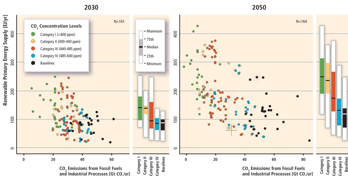
**Figure 1.1:** Global RE primary energy supply (direct equivalent) from 164 long-term scenarios as a function of fossil and industrial CO<sub>2</sub> emissions in 2030 and 2050 (IPCC, 2011). The colors represent categories of atmospheric CO<sub>2</sub> concentration level in 2100. The blue cross marks 2007 data. Although variations across scenarios are large, ambitious emission reduction targets imply a vast expansion of RE deployment.
