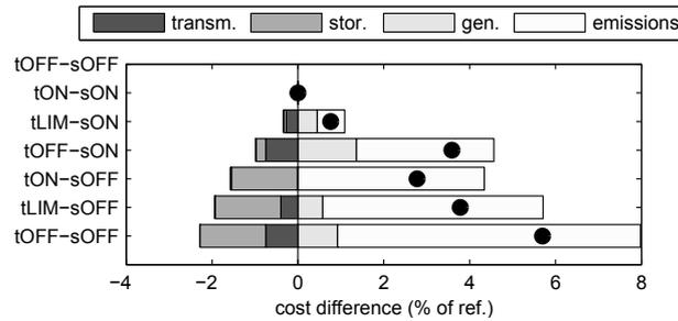
Figure 7: Decomposition of cumulated system costs, relative to the reference scenario ( $t_{ON-sON}$ ). Total costs are denoted by the black dots.
