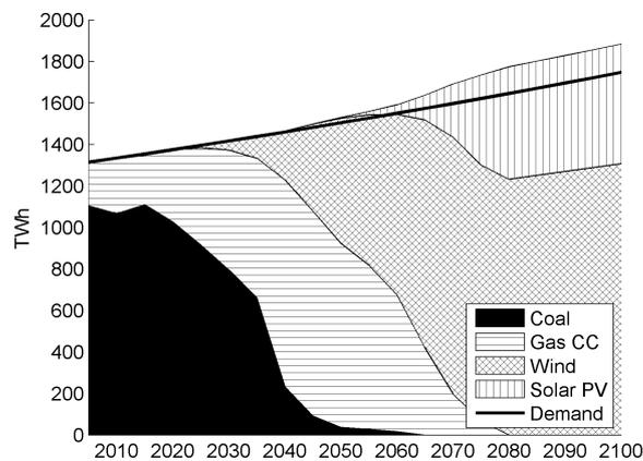
Figure 1: Generation mix and demand over time for the reference scenario. The differences between total generation and demand is due to transmission and storage losses. Curtailed power from RE sources is not shown.
