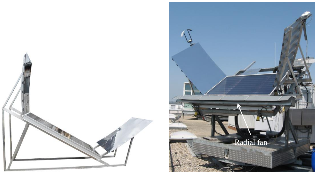
(a) RefleC 2 with the first variant of a mounting system with trapezoidal sheets
