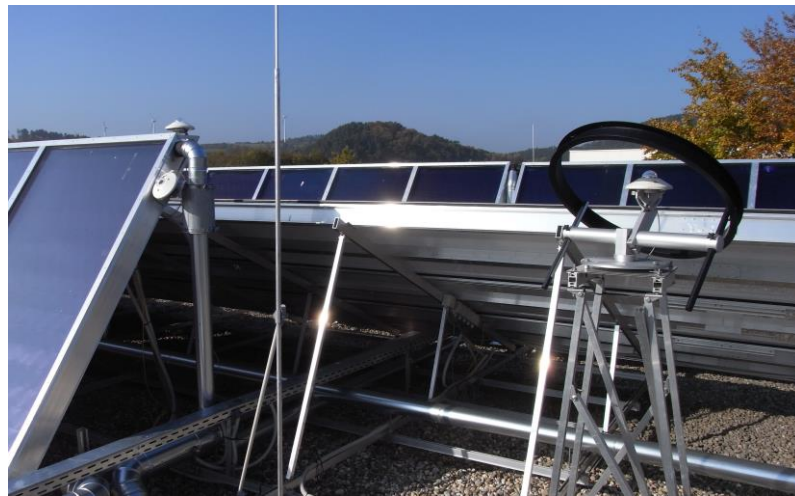
Figure 5.9: Positions of the three pyranometers applied for monitoring (2 CMP 11 and 1 CM 11, shadow band CM 121B). The hemispherical tilted irradiance G_t was measured in the aperture of the flat-plates (the RefleC aperture is in parallel and only centimeters behind, since it starts at the edge of the booster reflectors). The two other pyranometers measure horizontal hemispherical irradiance G and horizontal diffuse irradiance G_d . The axis of the shadow band was positioned east-west and the band was adjusted manually twice per week to shade the sensor from beam during the whole monitoring phase.
