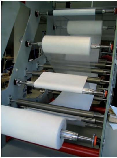
(a) Winding machine with material rolls [66]
