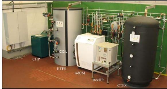
Figure 1. Microscale trigeneration lab at INES. From left to right: wall mounted Electric Switch Board (ESB), green coloured Combined Heating and Power (CHP), Electric Heating Coil (COIL), Hot Thermal Energy Storage (HTES), Adsorption Chilling Machine (AdCM), Reversible Heat Pump (RevHP), Cold Thermal Energy Storage (CTES)
