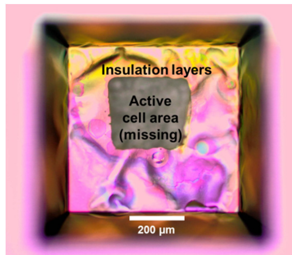
Fig. 8.1: Optical micrograph of a structure with a SiO 2 /Si NC layer of the most optimized run at the end of the fabrication process. The active cell area was torn out of the membrane exactly along the rim of the insulation layers (A and B). The Figure was adapted from [197].
